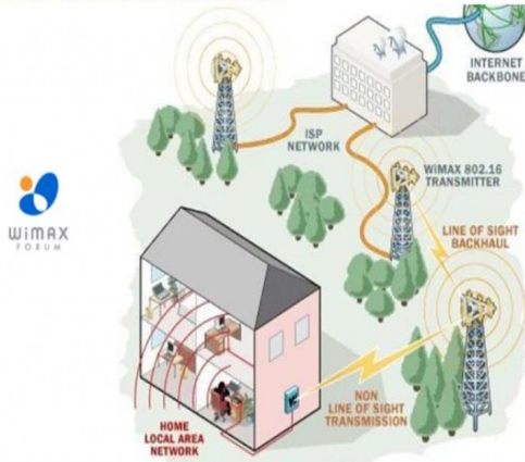
Figure 2.1 Fixed WiMAX Architecture
